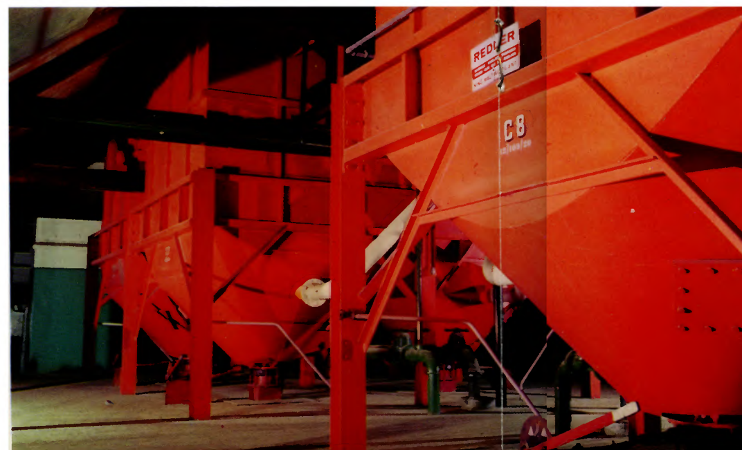
Left: Special ventilated type steeps.
