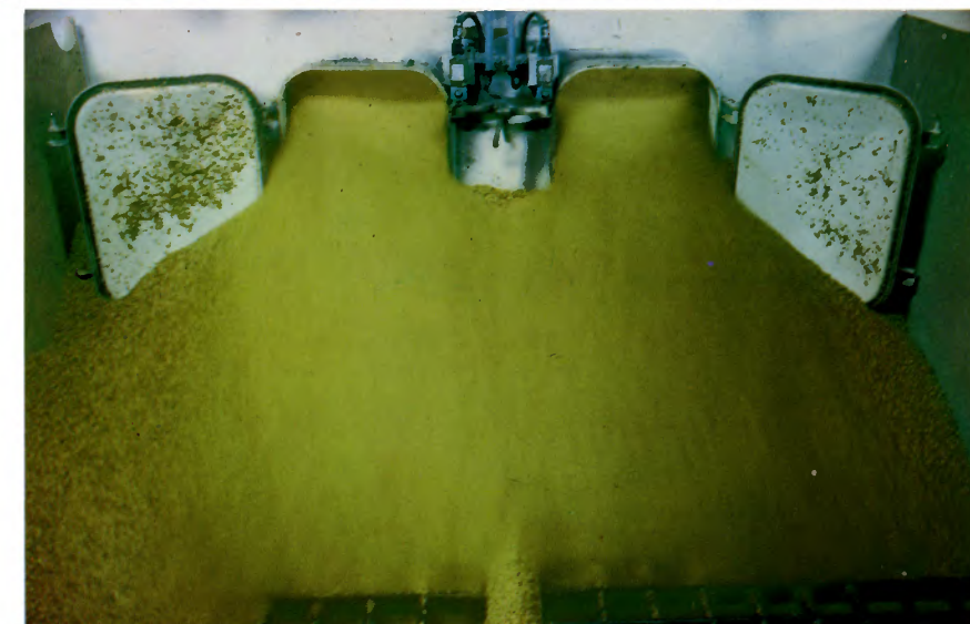
Left: Special ventilated type steeps.
