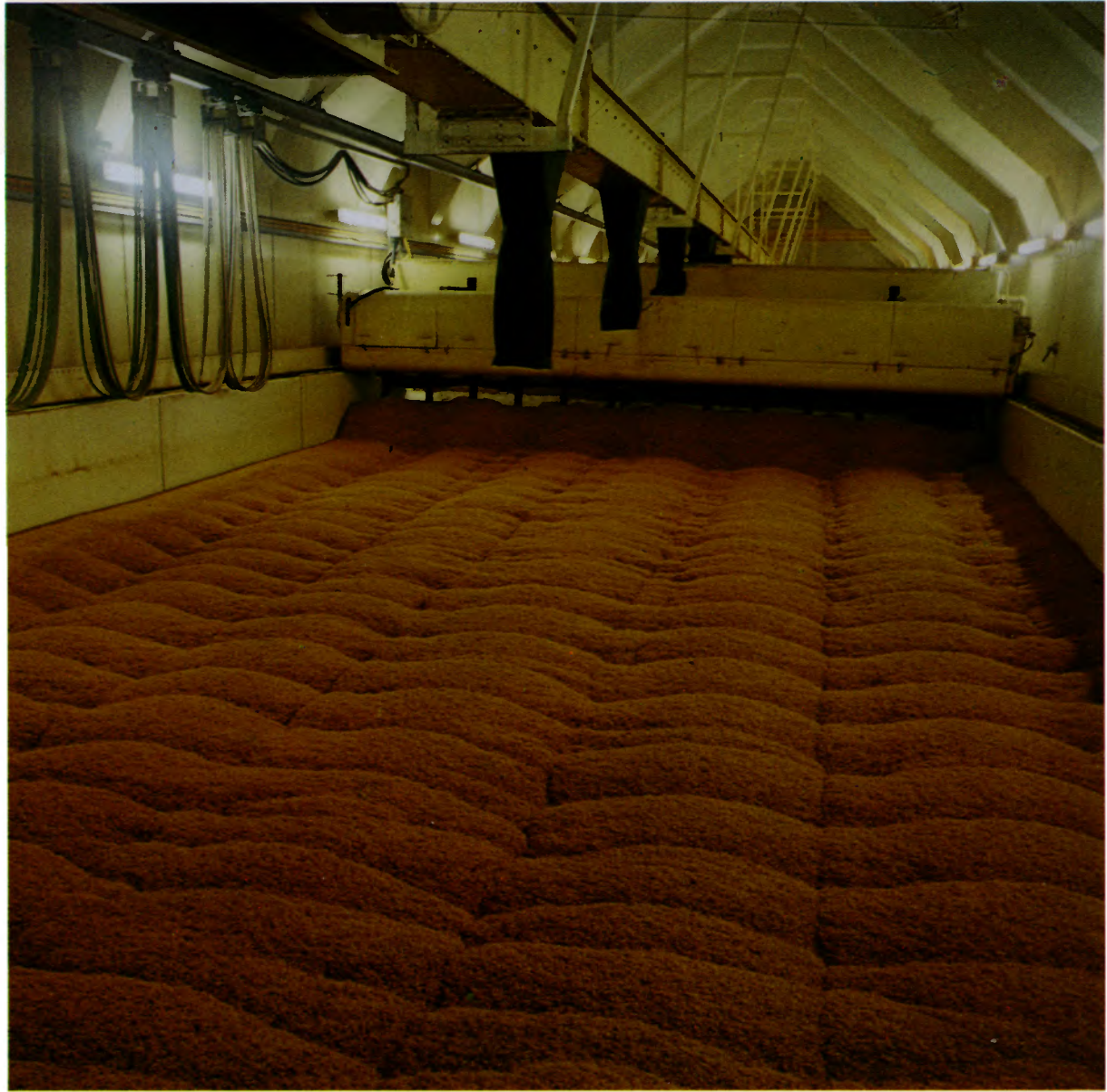
Bottom Right: Holding bin for malt-in-culm.
