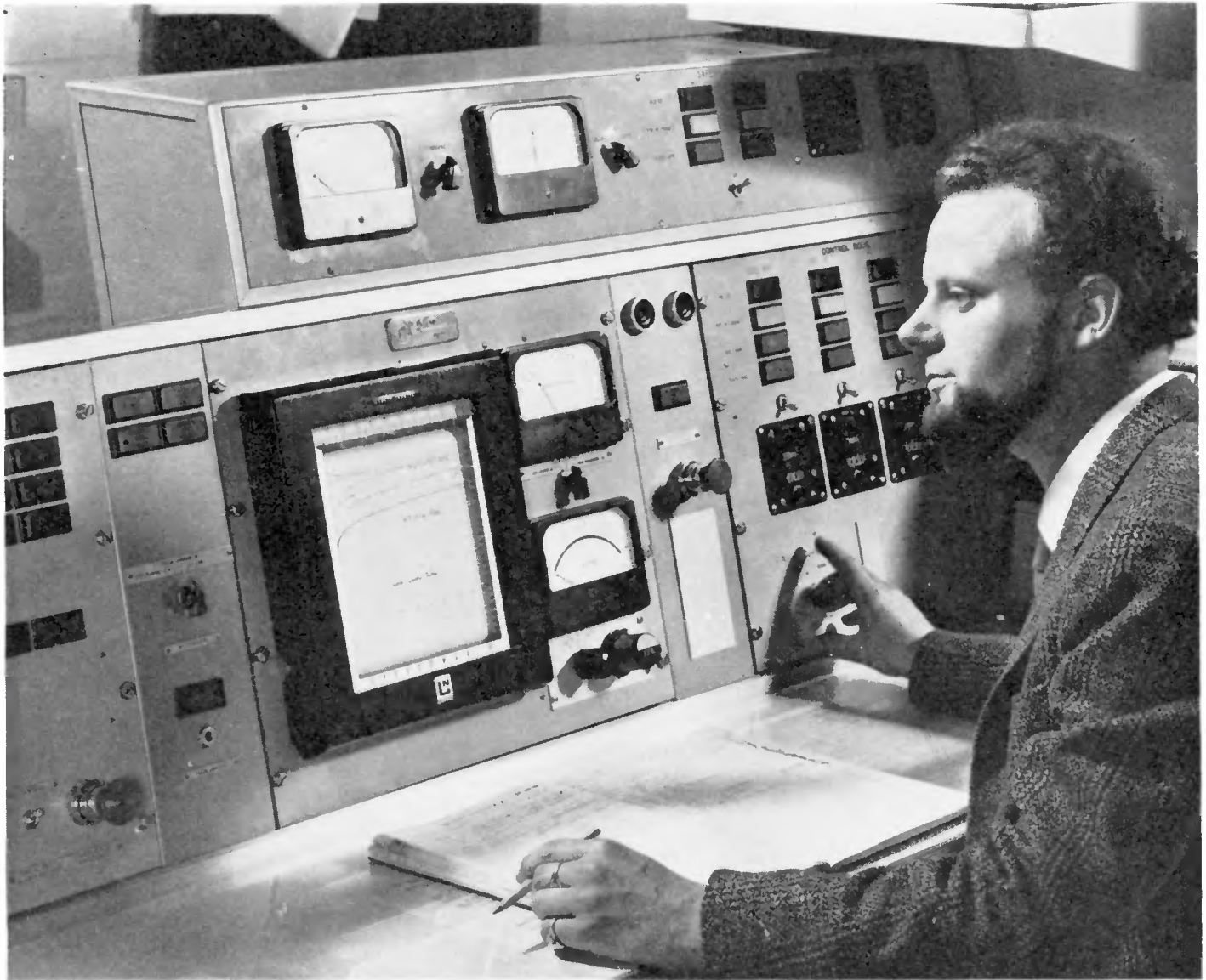
Operating console of the zero energy critical reactor facility. The flexible design of the facility allows rapid assembly of a wide variety of reactor cores.
