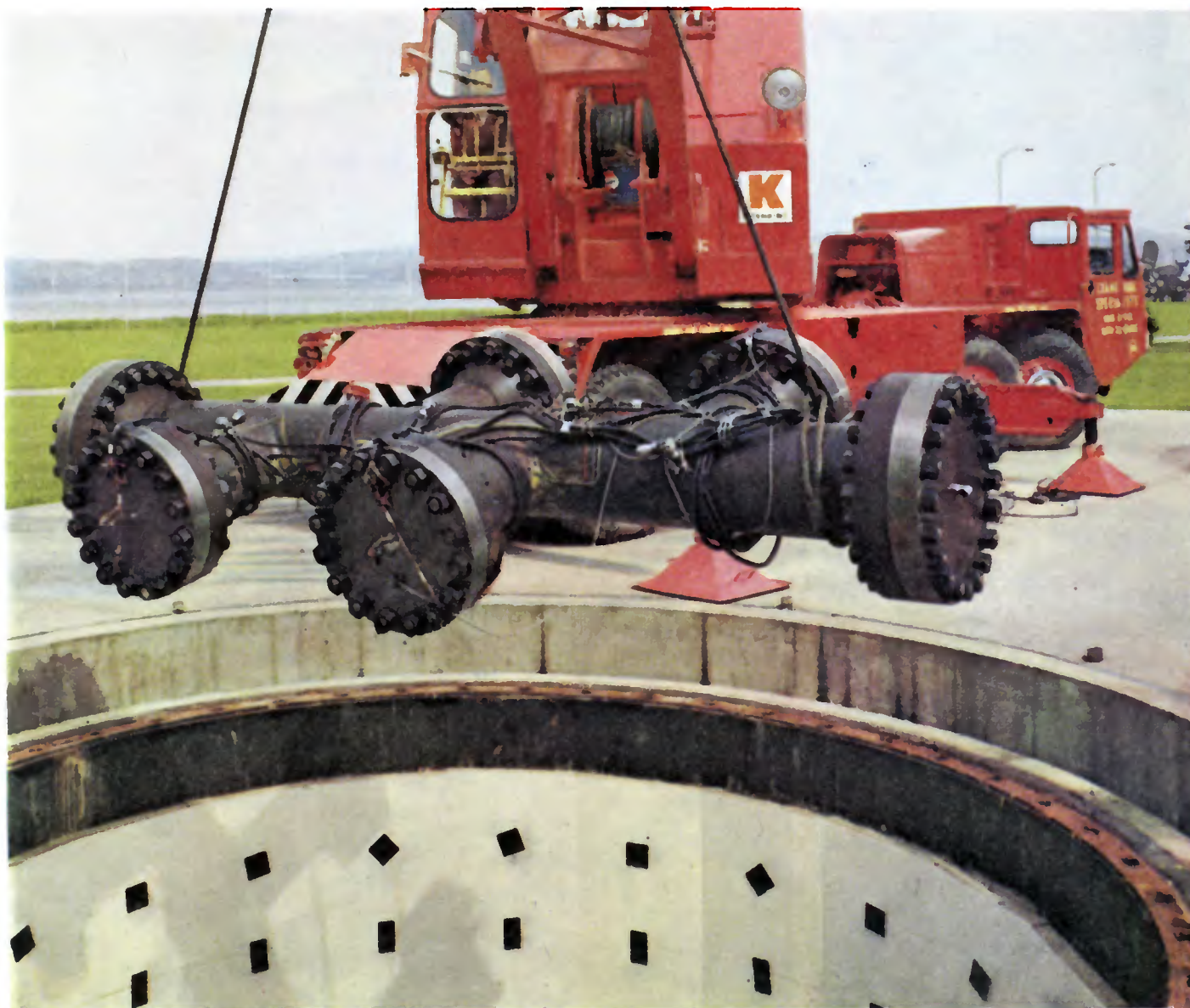
Large experiment on cylinder/cylinder interactions to confirm theoretical design predictions
