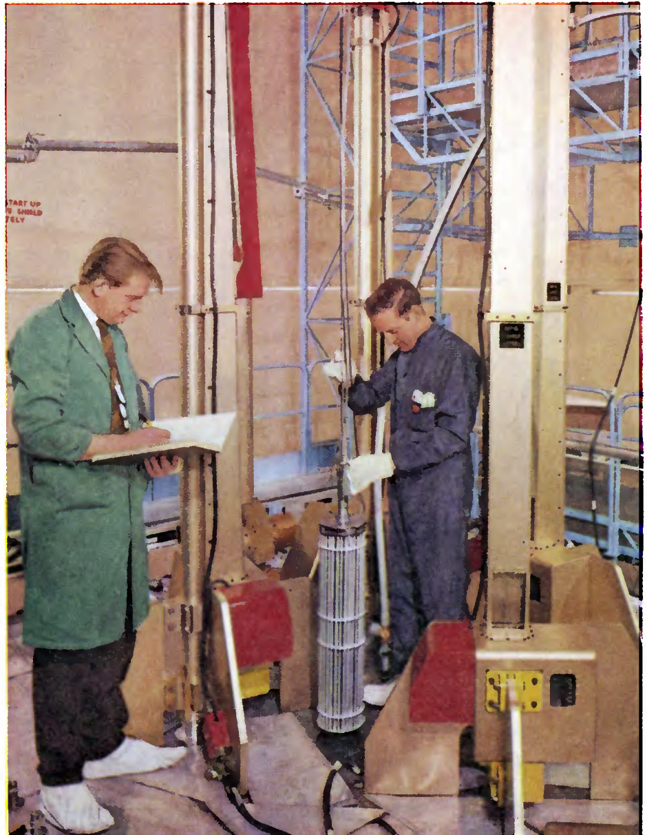
Experimental fuel being loaded into a zero energy assembly simulating an AGR reactor core. Results are used to test reactivity predictions
