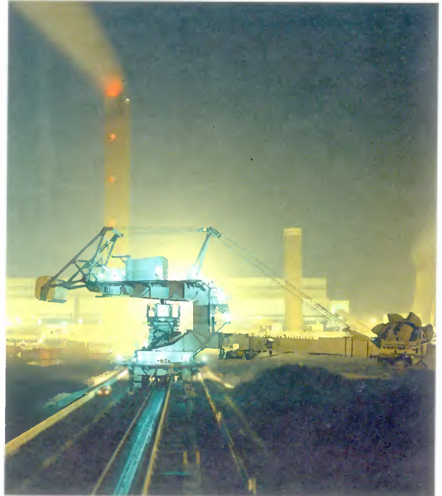
View from the coal stockyard of one of the two bucket-wheel machines at Drax power station. Each machine can handle 3000 tonnes of coal an hour.
