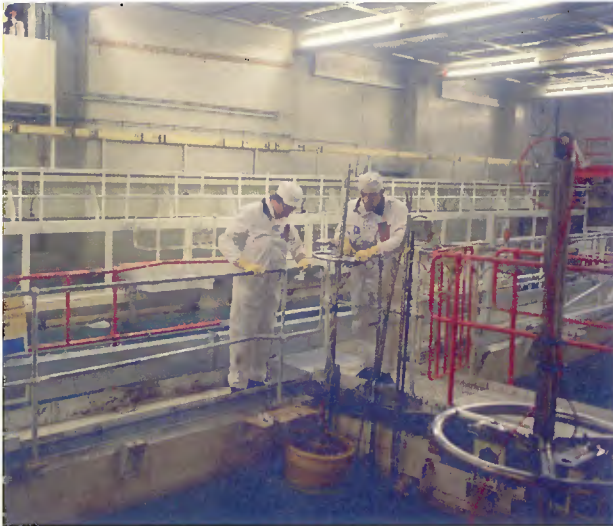
Tongs are used to place the elements into a skip.
