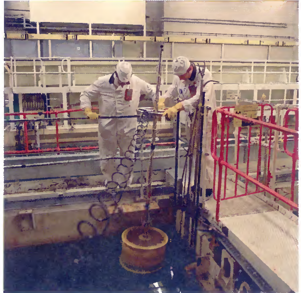
Tongs are used to place the elements into a skip.
