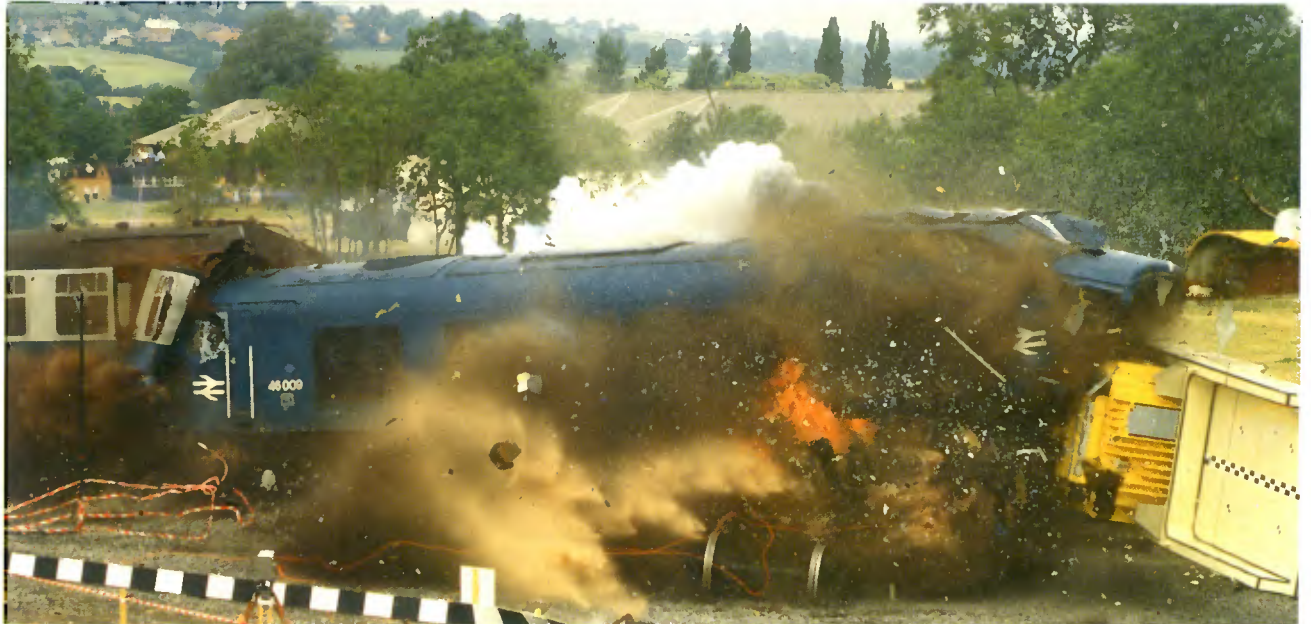
In a demonstration to show the strength of the fuel flask, a television audience of millions saw a diesel train travelling at 100 m.p.h. crash into a flask. The diesel locomotive was destroyed, but the flask was unscathed.
